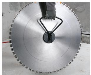
② Saw-blade flange, flush-cut
