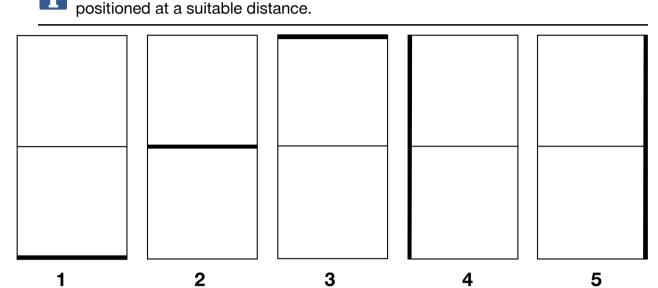
The illustration shows an example of the cutting sequence for a door opening with a dividing cut.
